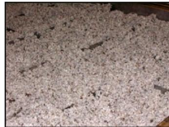
(d) Raw scrap natural rubber provided by B TECH Industry for producing skim block rubber
