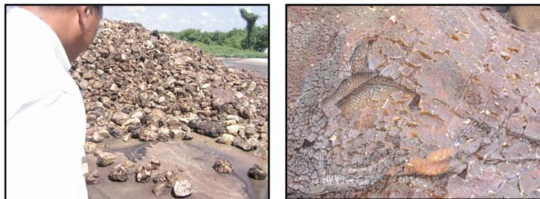
(a) Unclean scrap rubber and low grade ribbed smoked sheet rubber as raw natural for producing STR20 block rubber
