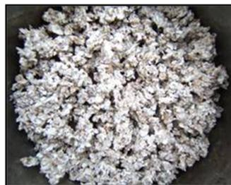
(c) Raw scrap natural rubber (after cleaning) provided by the Southland Resource Factory for producing STR20 block rubber
