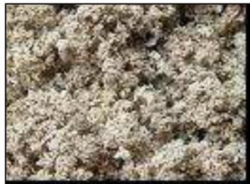
(b) Scrap rubber from wastewater of rubber latex factory as raw natural rubber for producing skim block rubber
