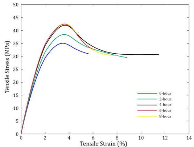
Figure 7. Stress-strain curves of specimens post-cured at various period
