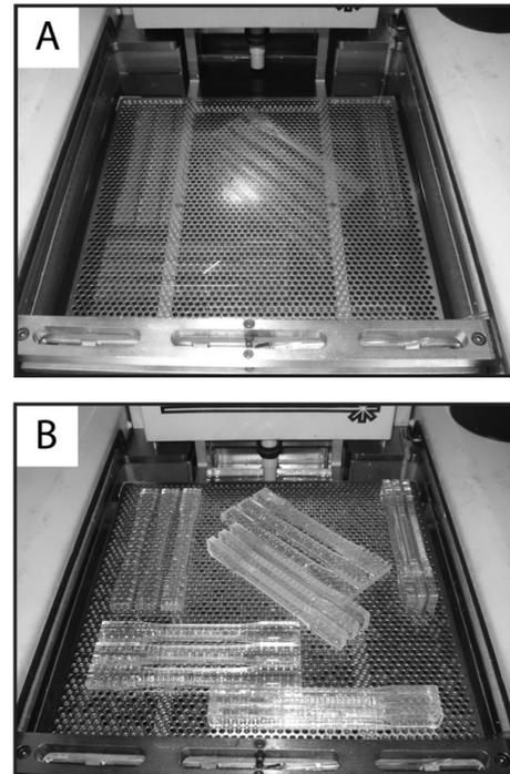
Figure 2. Fabrication of specimens, (A) during SLA process and (B) finished specimens
