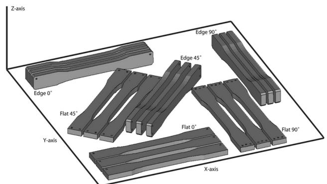
Figure 4. Build orientation
