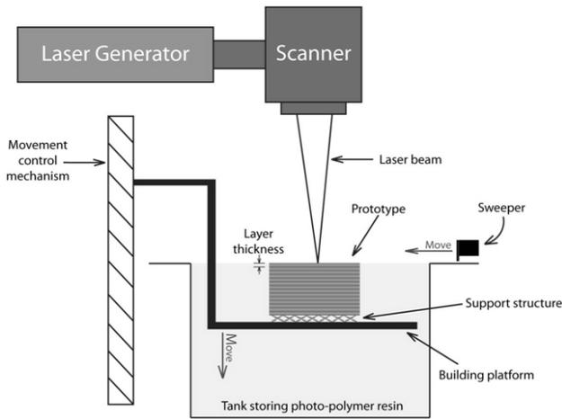
Figure 1. Stereolithography process
