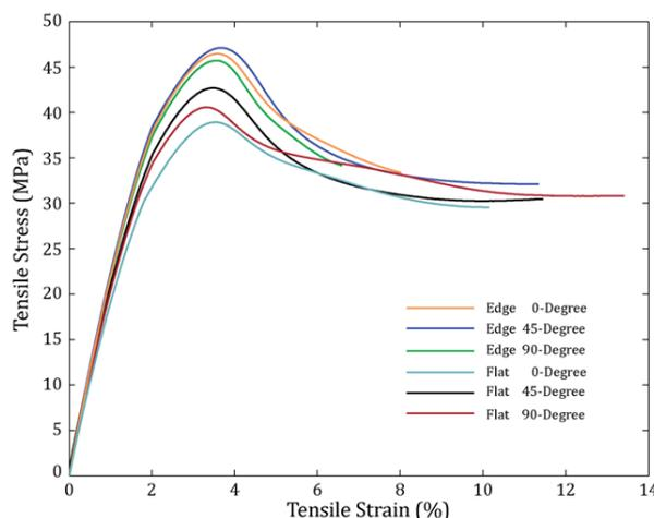
Figure 6. Stress-strain curves of specimens from different build orientation
