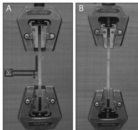
Figure 5. Tensile test, (A) Set up and (B) Failure of specimen
