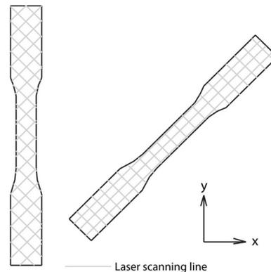
Figure 3. Cross-hatching laser scanning strategy
