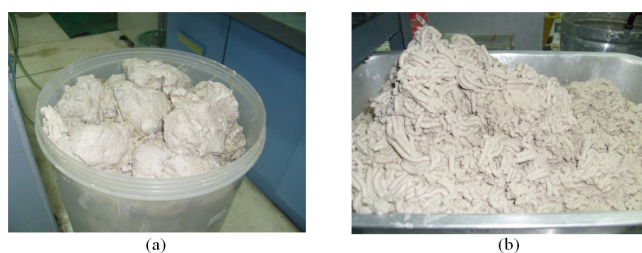
Figure 1. Waste latex sludge before (a) and after grinding (b).
