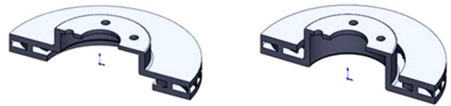
Figure 8. Front-vented brake disc (left) and back-vented brake disc (right).
