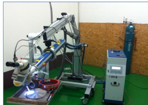
Figure 2. Nd-YAG Laser equipment.
