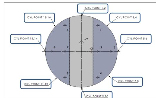
a) Measurement points for cylindrical diameter and roundness estimation.
