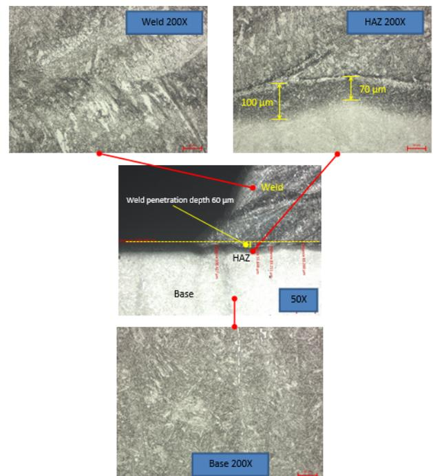
Figure 10. Microstructure of laser welded specimen No.1 at Weld, HAZ, and Base.
