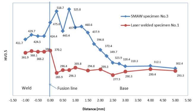
Figure 13. Micro hardness profiles of laser welded specimen No.1 and SMAW specimen No.3.
