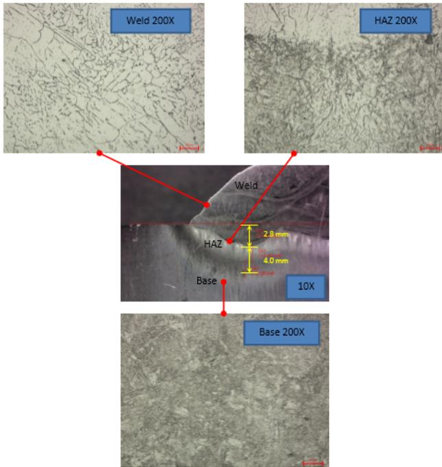
Figure 11. Microstructure of SMAW specimen No.3 at Weld, HAZ, and Base.
