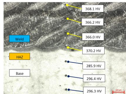
a) Laser welded specimen No. 1.
