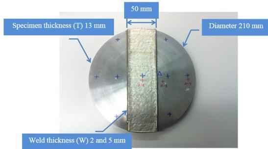
a) Laser welded specimens for thicknesses of 2 and 5 mm.
