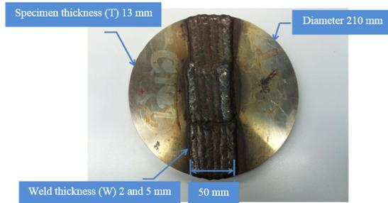
b) SMAW welded specimen for thickness of 5 mm.
