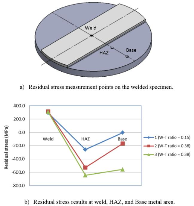
Figure 7. Residual stress results for laser welding specimen No.1 (W-T ratio = 0.15) and No.2 (W-T ratio = 0.38) and for SMAW specimen No.3 (W-T ratio = 0.38).
