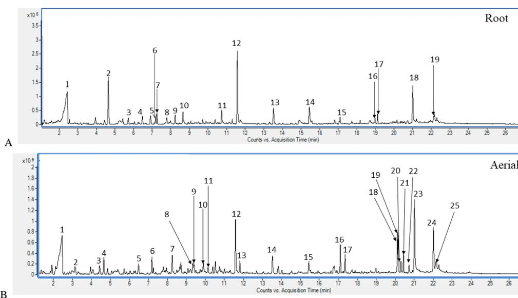
Figure 2. TIC from headspace GC-MS analysis of A) root part, and B) aerial part of *C. lappacea*. The peak numbers correspond to those in Tables 3-4.
