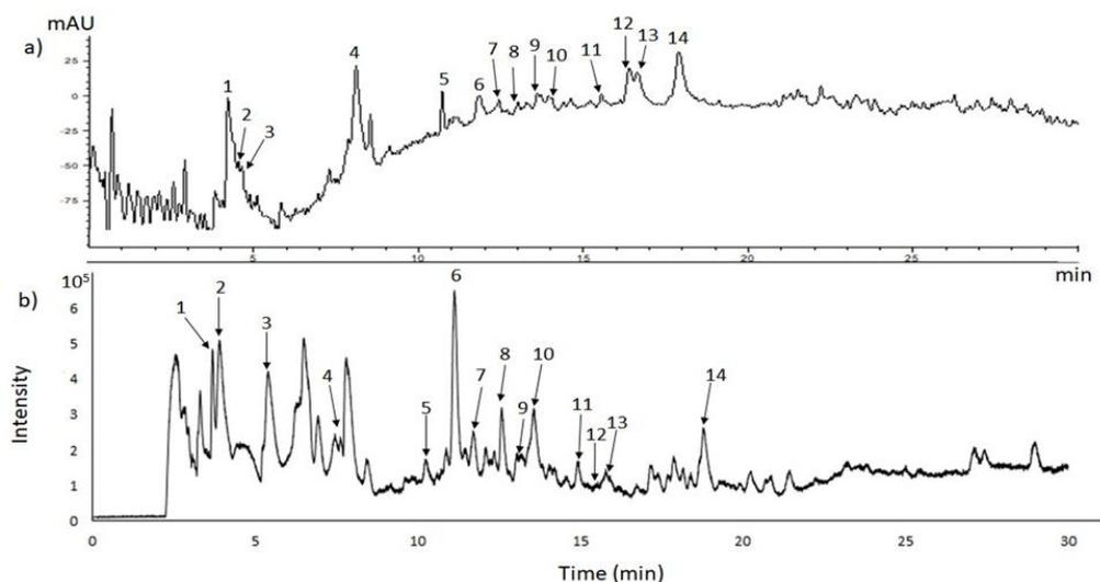
Figure 1. Separation of antioxidant compounds from 50% ethanol extract of *C. lappacea* performed by LC-ESI-QTOF-MS coupled with DPPH assay. (a) Chromatogram from antioxidant activity detector set at 515 nm. (b) The total ion current (TIC) output from the LC-ESI-QTOF-MS in negative mode
