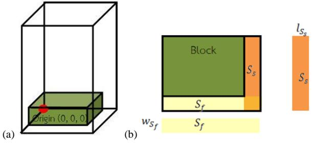
Figure 4. (a) Putting a block in *R* at the origin. (b) The free space on the side of block ( $S_s$ ) and the front of block ( $S_f$ ).  $W_{S_f}$  and  $l_s$  are width and length, respectively, of the free space on the side of block.
