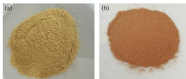
Figure 1. Mixed rare earth catalysts precipitated at pH 12 and stirring rate of 400 rpm (a) before calcination, and (b) after calcination at 300 °C for 3 h.
