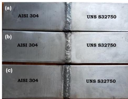
Figure 1. Dissimilar weldments of UNS S32750 and AISI 304 joined by using (a) ERNiCrMo-4, (b) ERNiCrMo-3 and (c) ER309L fillers
