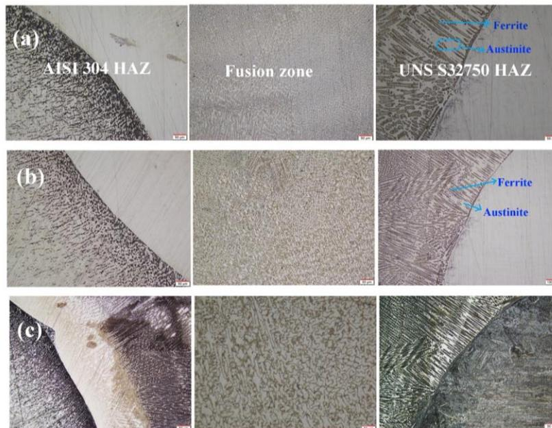
Figure 8. Microstructures of dissimilar weldments prepared with (a) ERNiCrMo-4, (b) ERNiCrMo-3 and (c) ER309L fillers
