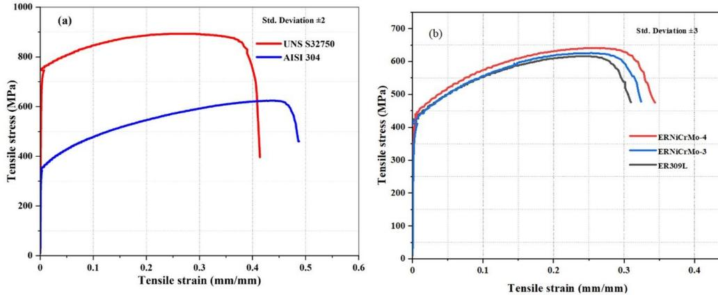
Figure 5. Stress-strain plots of (a) base metals, and (b) dissimilar weldments of UNS S32750 and AISI 304
