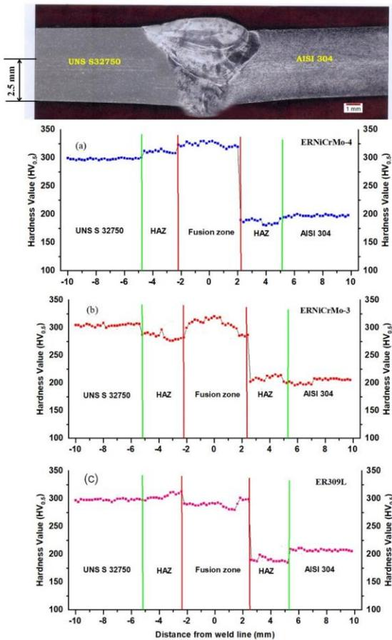
Figure 7. Hardness profiles of dissimilar weldments prepared with (a) ERNiCrMo-4, (b) ERNiCrMo-3 and (c) ER309L fillers.
