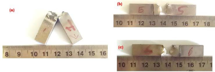
Figure 4. Impact test specimens of dissimilar joints joined by using (a) ERNiCrMo-4, (b) ERNiCrMo-3 and (c) ER309L fillers.
