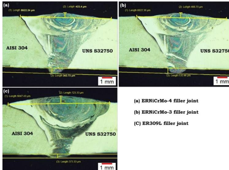
Figure 3. Macrostructures of dissimilar UNS S32750 and AISI 304 weldments prepared with three alternative filler wires.
