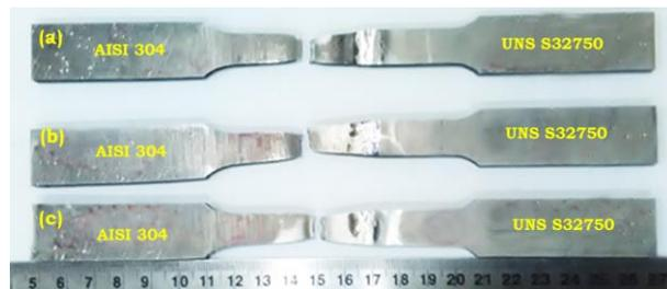
Figure 6. Tensile failure specimens of dissimilar weldments joined by using (a) ERNiCrMo-4, (b) ERNiCrMo-3 and (c) ER309L fillers.
