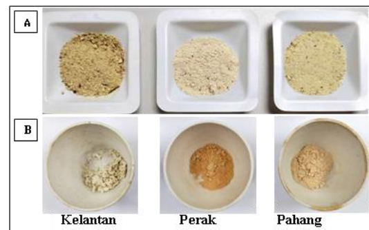
Figure 3. S. myosotiflora dried tubers in powder form (A) and after ashing at 550°C overnight for the total ash determination (B)
