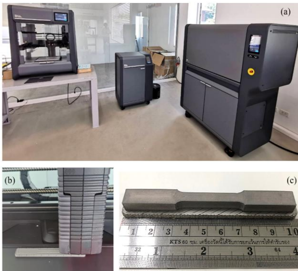
Figure 1. (a) The studio system of Desktop Metal at Thaisakol Group Co., Ltd., (b) build direction is horizontal, and (c) 3D printed specimen after sintering
