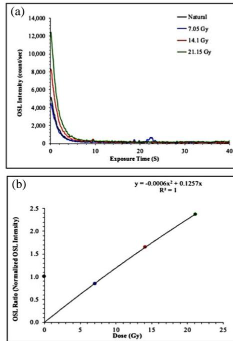
Figure 2. Representative OSL (a) decay curves and (b) growth curve of old sandy beach sample NK4, where N represents the natural (Natural = 6.78 Gy) (black dot) and single (blue dot), double (red dot), and triple regenerative doses (green dot), respectively.
